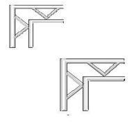
All Opti Trilite 200 series is connected together using aluminium spigot connectors and 2 x nuts & bolts inserted into ends of the fabricated sections
