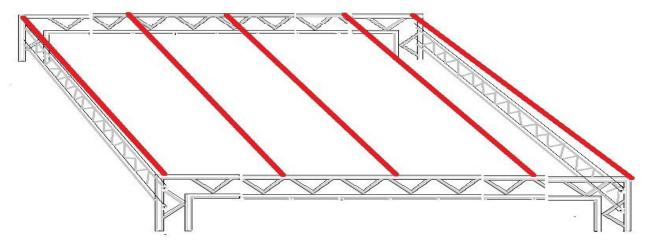
Ratchet straps are now attached to Opti Trilite 200 series frame, running from the front to the rear.
