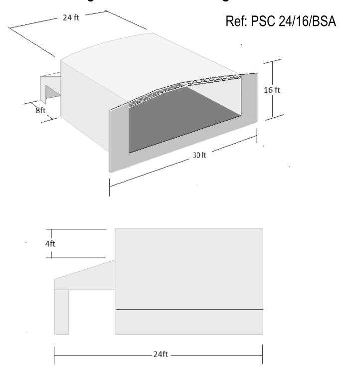
Total performance area 24ft wide x 16ft depth stage height 3ft, curved roof, and has a additional rear back stage area. This set up uses 12 x 8ft x 4ft Steel deck sections, which are bolted together. The OPTI Trilite 200 aluminium trussing makes up the canopy structure, upon which the PVC sheets are attached using bungee ties.
