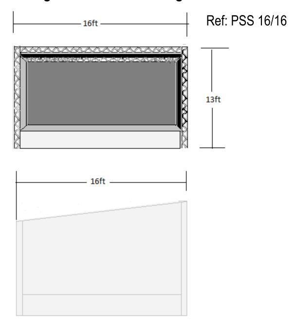
Total performance area 16ft wide x 16ft depth stage height 2ft, sloped roof.
