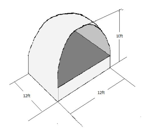
Total performance area 12ft wide x 12ft depth stage height 2ft, Arc roof.
