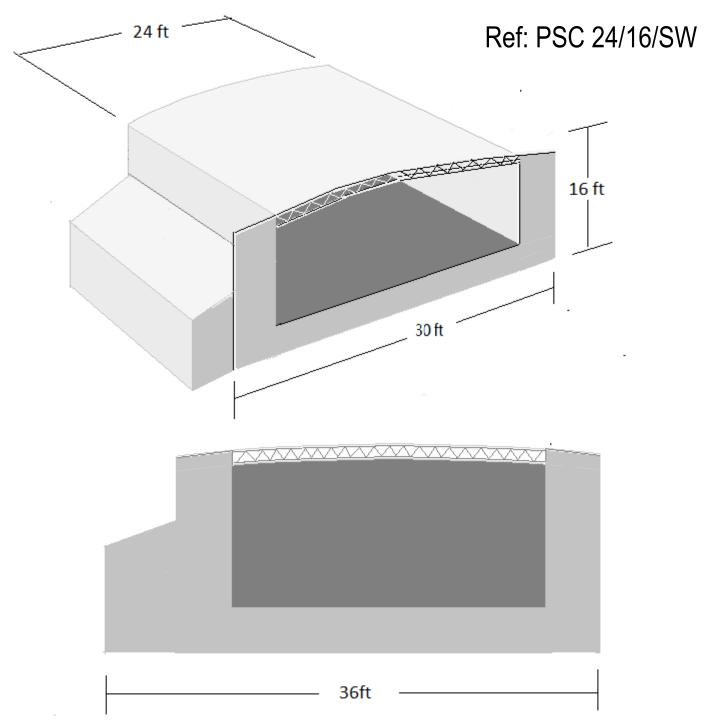
Total performance area 24ft wide x 16ft depth stage height 3ft, curved roof, and side wing area.
