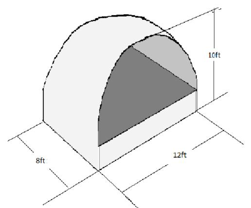
Total performance area 12ft wide x 8ft depth stage height 2ft, Arc roof.
